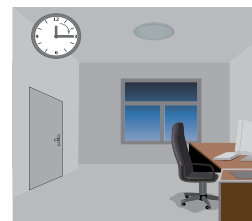
Light switches off automatically after the stand-by period elapses.
